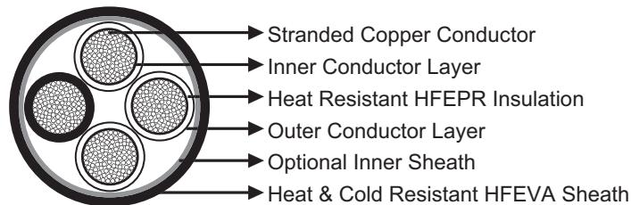
**Conductor:** Stranded tinned/bare copper, class 5 according to DIN VDE 0295 IEC 60228.
